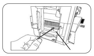
X Tighten the screws behind the fixing base plate of the fluorescent module to fix the fluorescence module on the microscope.
