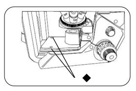
1 Adjust the coarse focusing screw to raise the objective lens, take out the two screw hole plugs on the bottom plate, loosen the screws with a hexagonal key, and take the bottom plate from the microscope.
