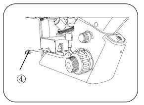
Push and pull the fluorescent rod to exchange different fluorescence channels.
