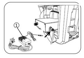
Plug in the power adapter cable and plug the other end of the power adapter into the power socket.
