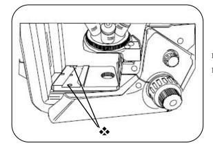
Push in fluorescent module fixed bottom plate on the microscope base, and the bottom plate is fixed on the microscope by tightening the screws.
