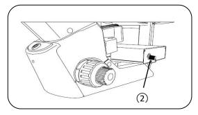
Turn the switch / brightness adjustment knob to hear the sound of "click", that is, the light source has been turned on. Continue to turn the knob to increase the brightness. Adjust the fluorescence to the appropriate brightness.
