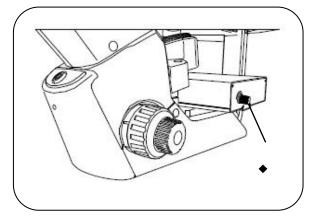
◆Clip the fixing groove of fluorescence module into the installed bottom plate track, and slowly push it into the microscope light path along the track.
