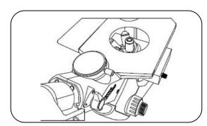
◆ Put the sample on the stage, switch to the "10x" objective lens, and adjust the thickness of the quasi focus spiral focusing.
